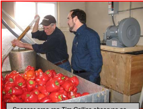
Spencer area rep Tim Collins observes as Foodshare's Steve Slipchinsky demonstrates how waste produce is moved into the tank. The Spencer Vortex® blower and starter in the background simplify the recycling process.
